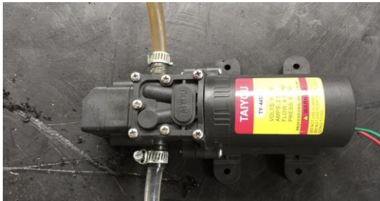
Fig 05: Diaphragm water pump (TAIYOU TY-44520)
