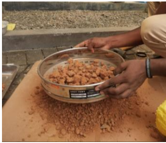
Figure 2.2 Gravel soil sieving by 37.5mm sieve
